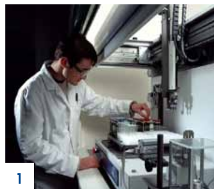
1-2. Analytical high-performance liquid chromatography (HPLCMS) system with a diode array detector and coupled to a mass spectrometer
