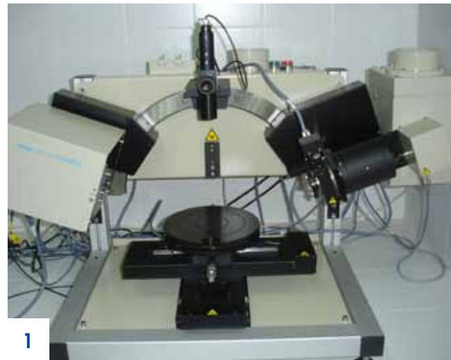
Mapping of a surface layer thickness obtained by ellipsometry
